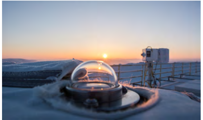
The Brewer spectrophotometer dome. The instrument is deployed around the world to measure ozone.
