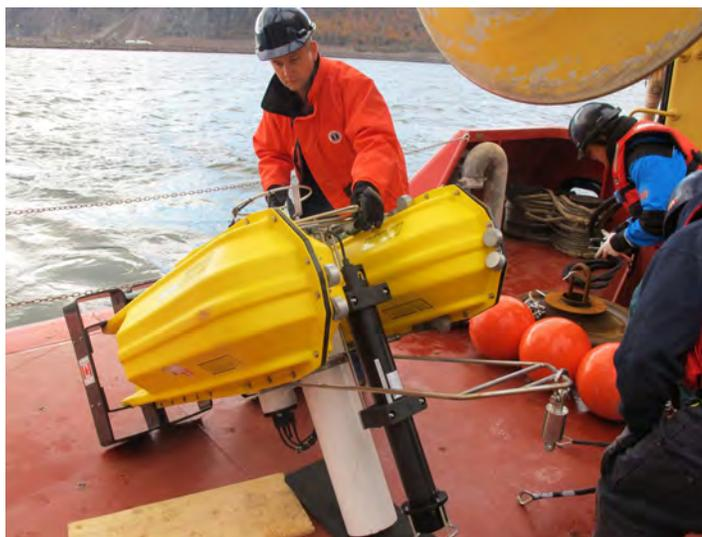
Figure 3: The ice draft node prepared for deployment.
