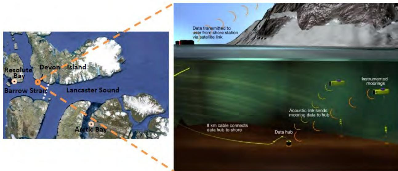
Figure 1. The configuration and location of DFO's real time ocean observatory at Gascoyne Inlet on the north side of the eastern Northwest Passage. The dashed line across the Strait east of the observatory location indicates the location of an instrumented mooring line maintained from 1998 until 2011.
