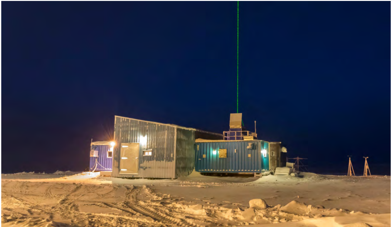
The CANDAC Raman Lidar (CRL) at the Zero-altitude PEARL Auxiliary Laboratory (0PAL) taking nighttime measurements of the high Arctic atmosphere (e.g. temperature, H 2 O).
