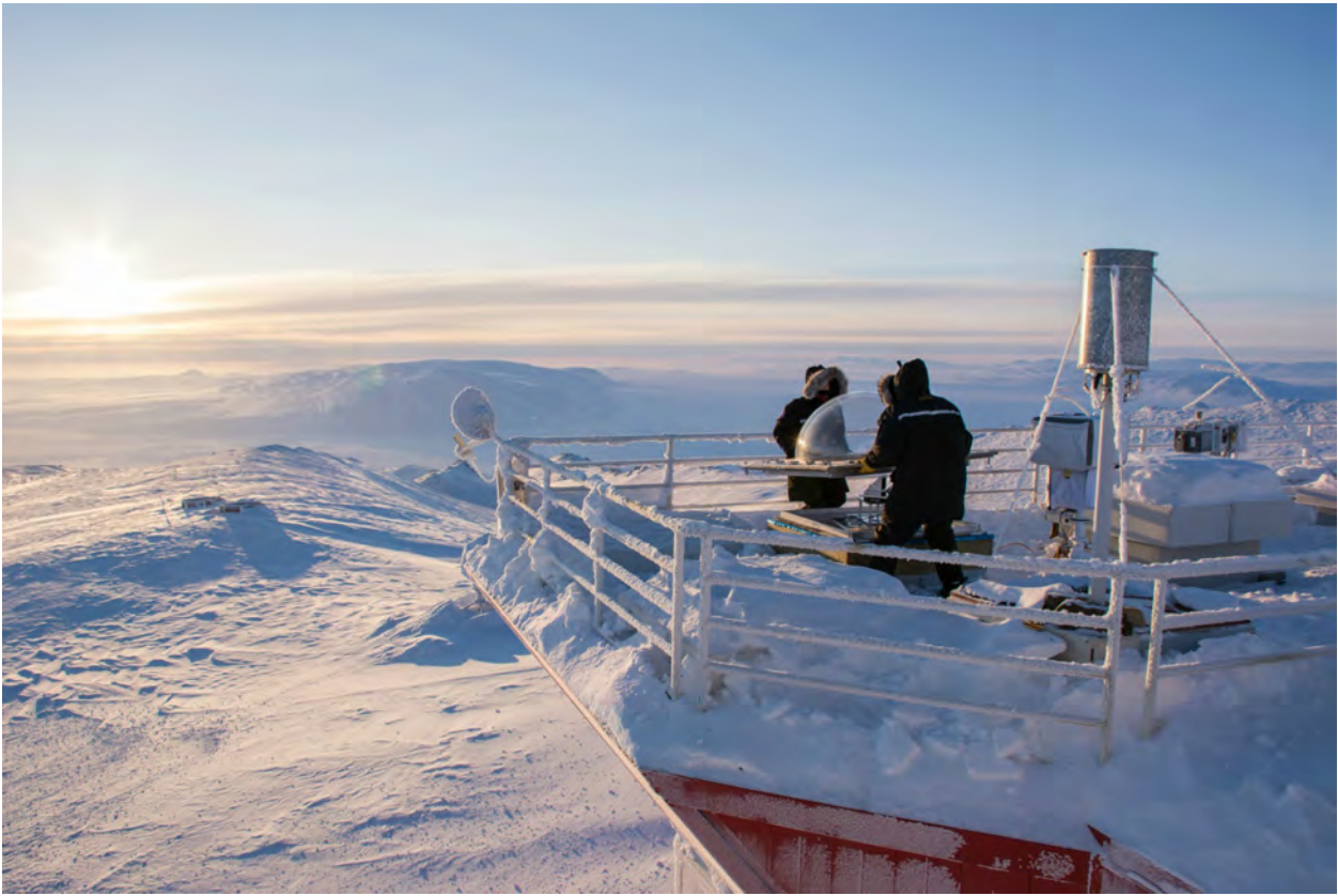
PEARL researchers open the dome of a sun tracking instrument on the roof of the Ridge Lab to perform maintenance.
